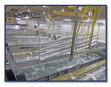
Architectural Anodizing combines science with nature to create one of the world's best metal finishes. Anodizing is the process of electrochemically controlling, accelerating and enhancing oxidation of an aluminum substrate. The anodizing process, because it is an integral part of the substrate, produces an oxide film that is uniform, hard and protects the rest of the aluminum substrate from
