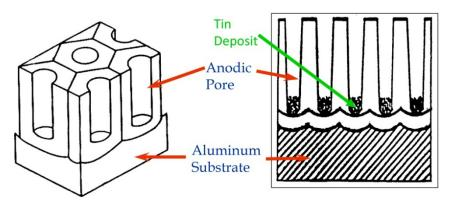
Note that tin is deposited at the bottom of the anodic pore. The intensity of the color depends on the amount of tin deposited
