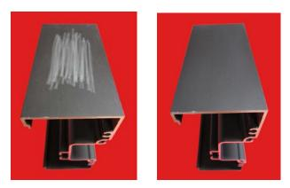
The first illustration shows the anodized aluminum scratched multiple times by a nickel. The second image shows the aluminum after being wiped with a wet cloth. The scratch residue comes right off and the aluminum is completely unharmed.
