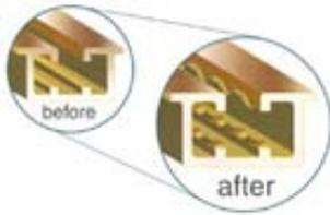
When the pour and debridge process is completed and the window is assembled there is no aluminum contact exterior to interior. Thus, transfer of temperature is interrupted, resulting in an energy-efficient, insulating thermal barrier. Temperatures of  $-100^{\circ}\text{C}$  will not transfer with pour and debridge thermal barrier in an aluminum frame-neither will hot temperatures. [View AAMA specifications and material properties](#)
