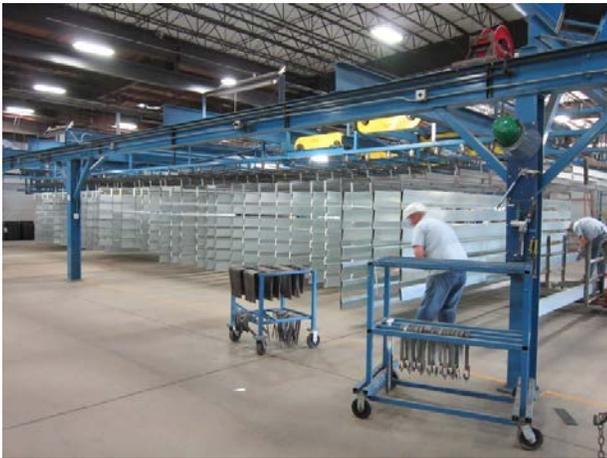
Products are racked horizontally on a 960-foot long overhead conveyor that travels up to 24 feet per minute. All parts have unique racking methods based on the exposure of the material. Racking is a critical step in the process to ensure the automated spray bells and the painters can get good coverage in all exposed areas.
