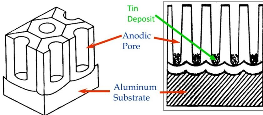
Note that tin is deposited at the bottom of the anodic pore. The intensity of the color depends on the amount of tin deposited
